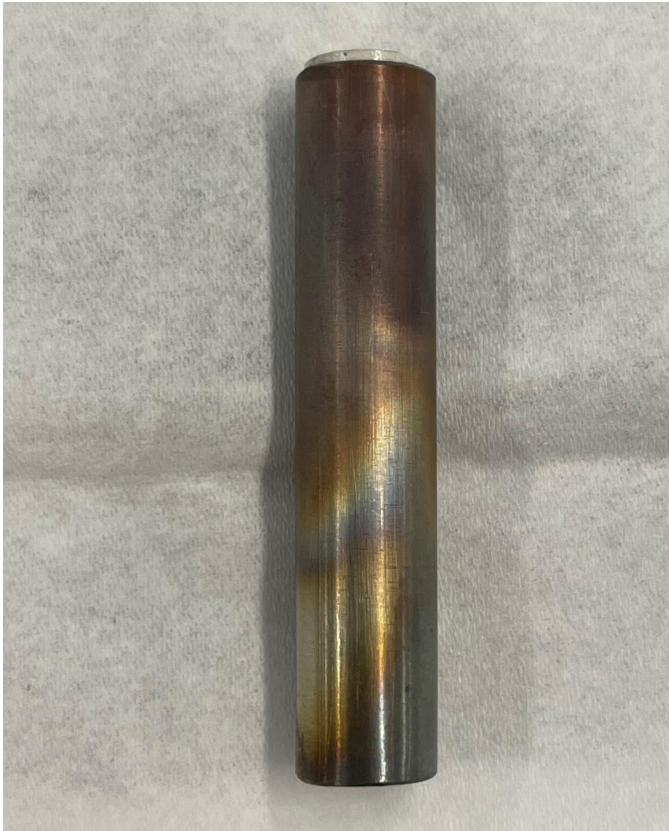
Mullite pellets glued inside oxidized (sst) cladding
