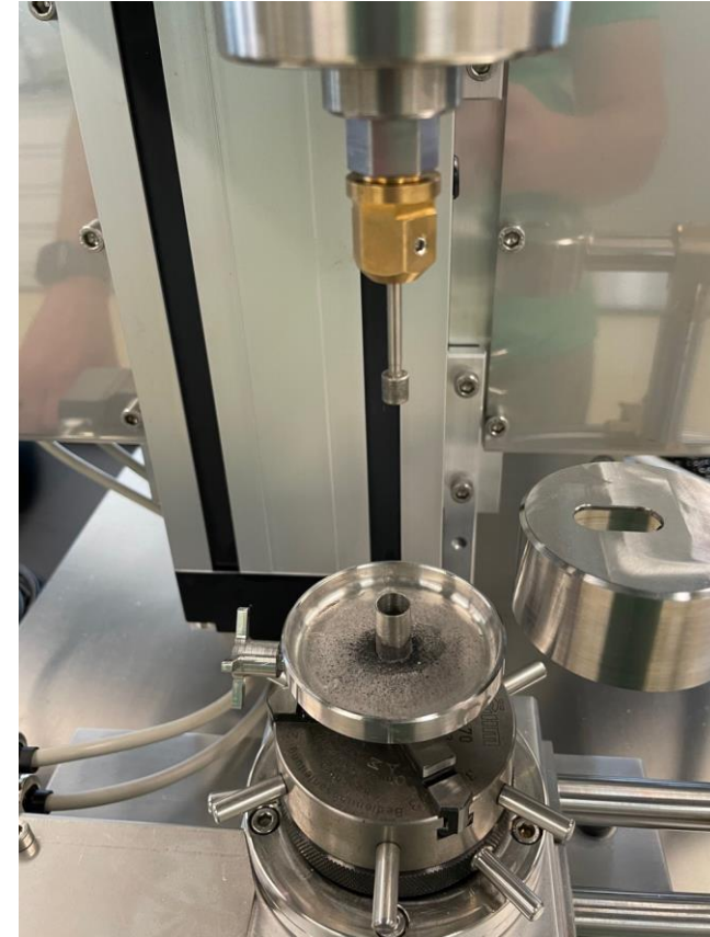
Top pellet removed and oxidation cleaned from inner and outer surfaces of the cladding (this is prep for welding)
