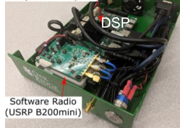
All commercial components + ORNL DSP (data-2-info) & communication to the enterprise network
