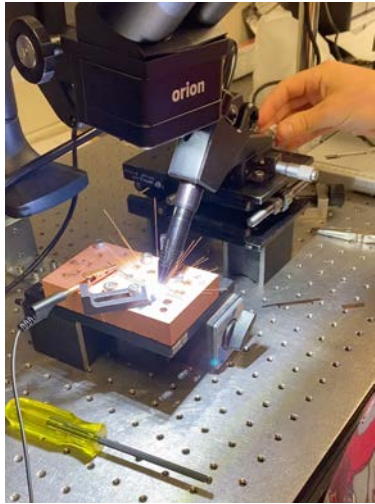
TIG Micro-welding SS316 sensor joints
