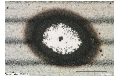
Localized dynamic failure of sensor using laser ablation
