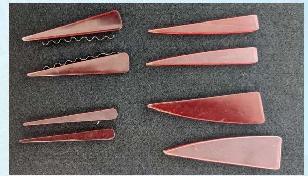
Flat Tapered and Profiled 3-D-printed Wedges
