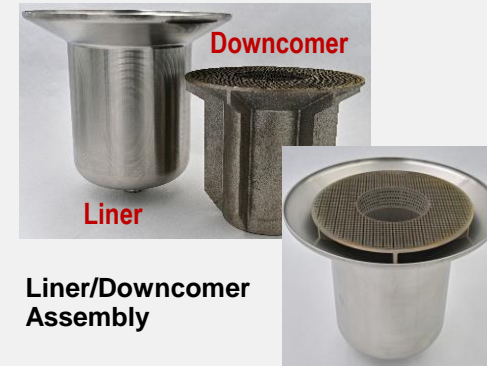
AddUp BeAM Modulo 400 DED Liner: 316L SS Size: 400 x 400 x 650 mm †
