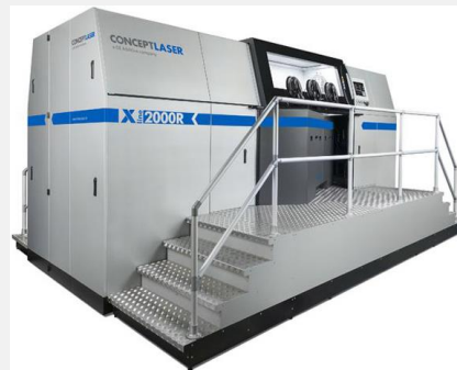
GE Concept Xline 2000R LPBF Liner & downcomer: In 718 Size: 800 x 400 x 500 mm †
