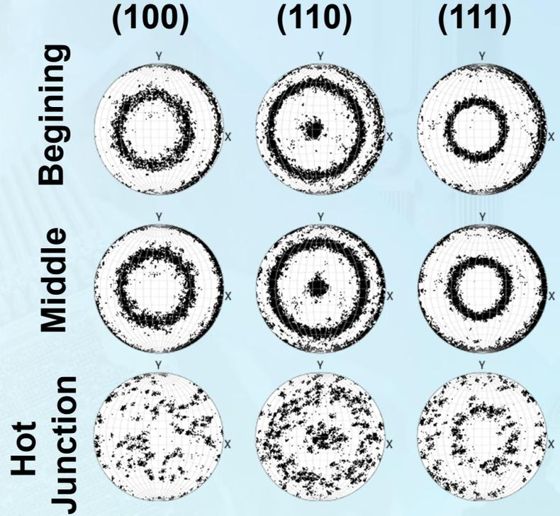
**Findings:** The HTIR-TCs maintained a 110//drawing axis fiber texture after Joule heating and a subsequent hold for 50 hours at both 1250 and 1450 °C.
