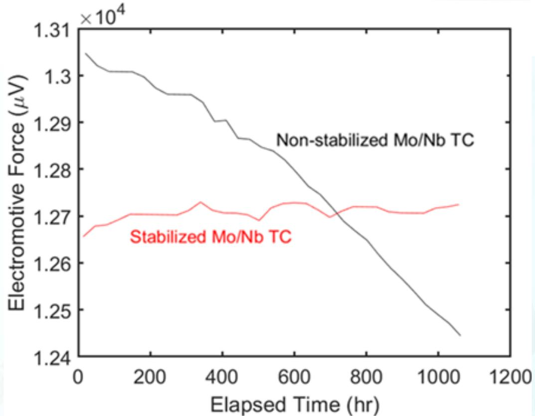
Signal measured by Mo/Nb thermocouples during 1000-hour 1100 °C test [4].
