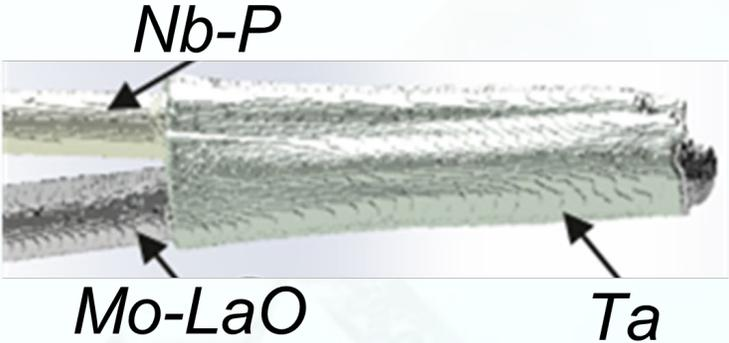
Joule heating model of HTIR-TC hot junction cross-section in COMSOL<sup>1</sup>
