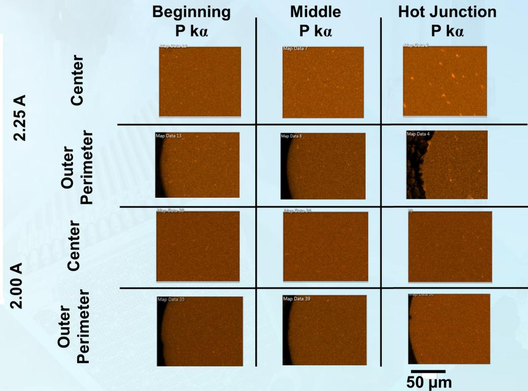
**Findings:** Joule heating resulted in coarsening of the Nb<sub>3</sub>P phase within the Nb-P thermoelement.
