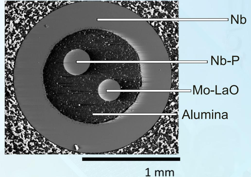
SEM micrograph of HTIR-TC cross-section
