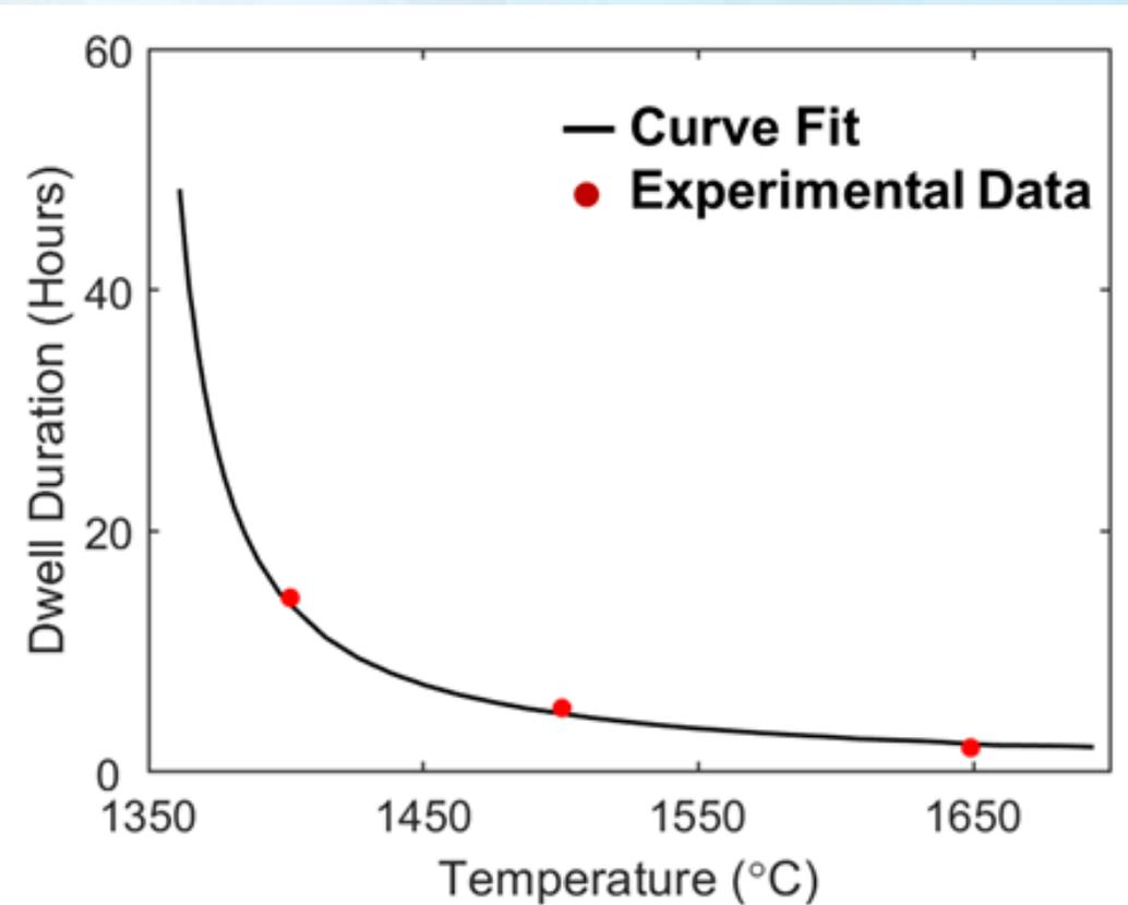
Hours to stabilize as a function of heat treatment temperature for HTIR-TCs.
