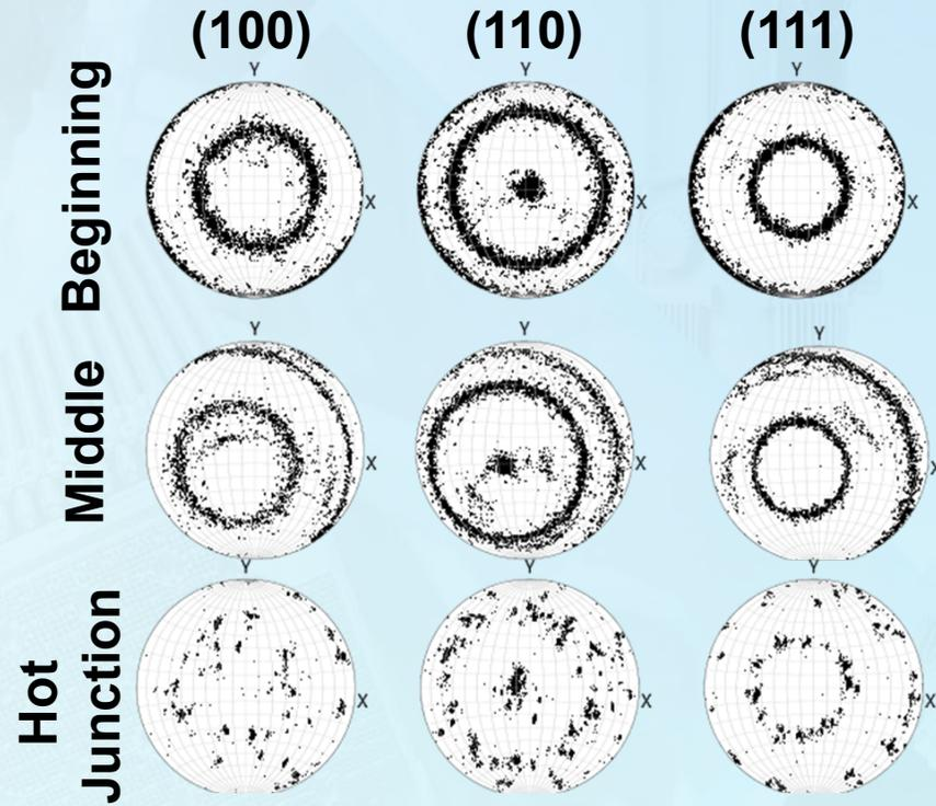
**Findings:** The HTIR-TCs maintained a 110//drawing axis fiber texture after Joule heating and a subsequent hold for 50 hours at both 1250 and 1450 °C.
