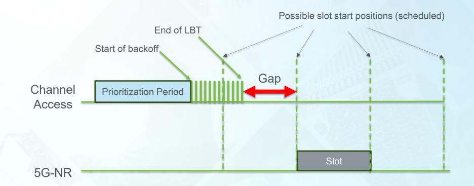
Fig.: 5G-NR : Gap between Slot start boundary and End of LBT procedure
