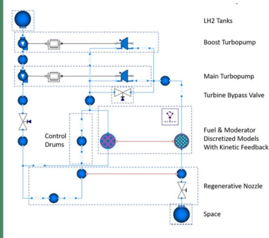
• 1-D flow, 2-D r-z solid fuel and moderator with appropriate lumped mass simplifications
