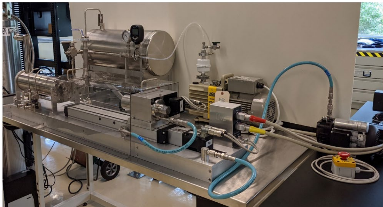
Cryo-drilling unit with vacuum pumps and guards in place
