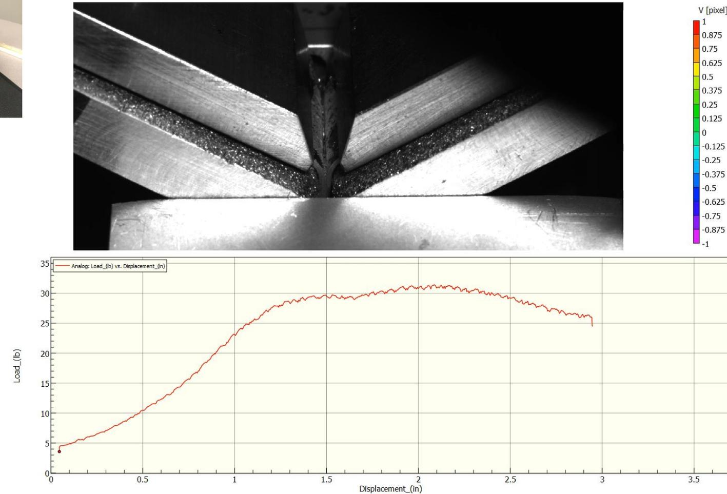
Ref.: Standard Test Method for Peel Resistance of Metal Sheets Joined by High Strength Bonds, ASTM B1021.
