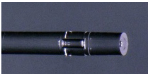
Photograph of the active compensation prototype sensor using cascaded Fabry-Perot cavities.
