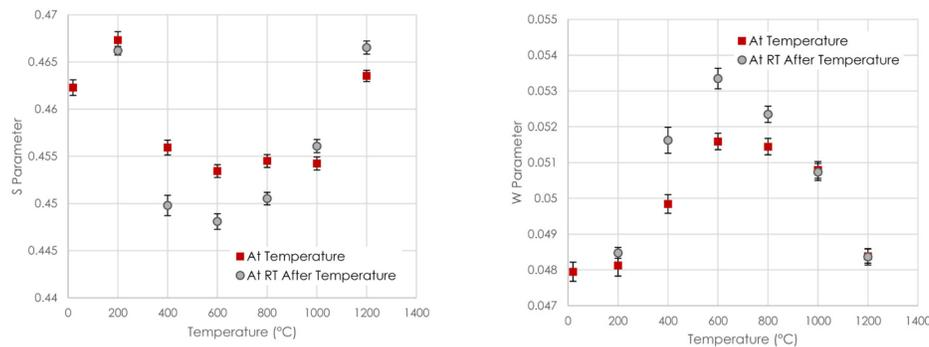
Figure 1. S and W parameters of the Ga<sub>2</sub>O<sub>3</sub> sample, as a function of temperature.
