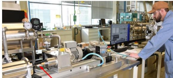
**Preparing to start cryo-drilling of a surrogate fuel rodlet**
