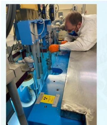
Installing sensors in NRAD
