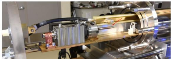
**Lining up tungsten electrode prior to welding**
