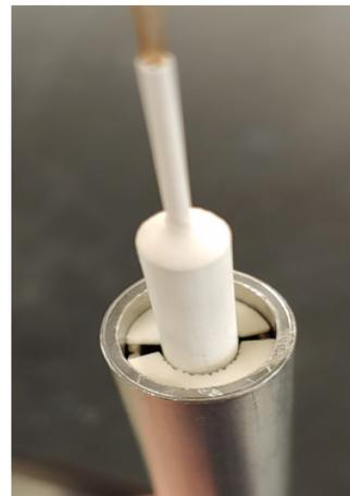
Figure 2. Improved OFBGT with a slightly thicker (double wall) outer sheath to house the fiber.
