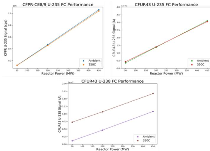
Figure 2. Performance of all three fission chambers irradiated at OSURR.
