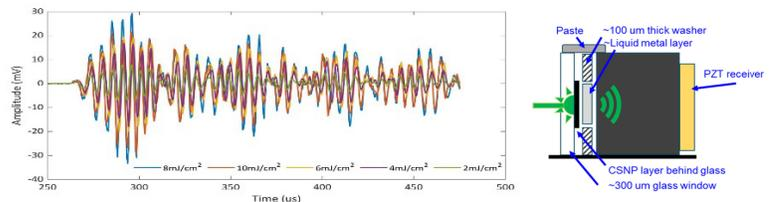
Figure 2. Left: LM-CSNP fluence test results. Right: transducer diagram.
