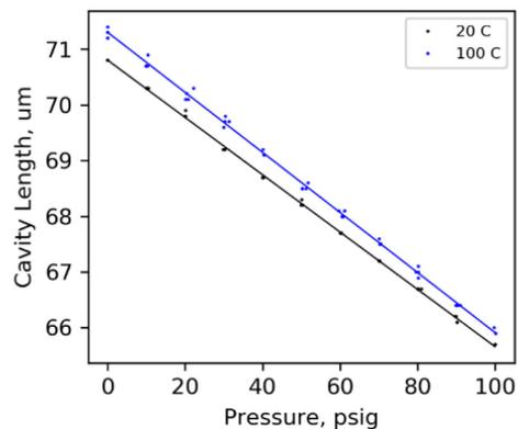
*Figure 2. Experimental results from testing the sensor performance at elevated temperatures.*
