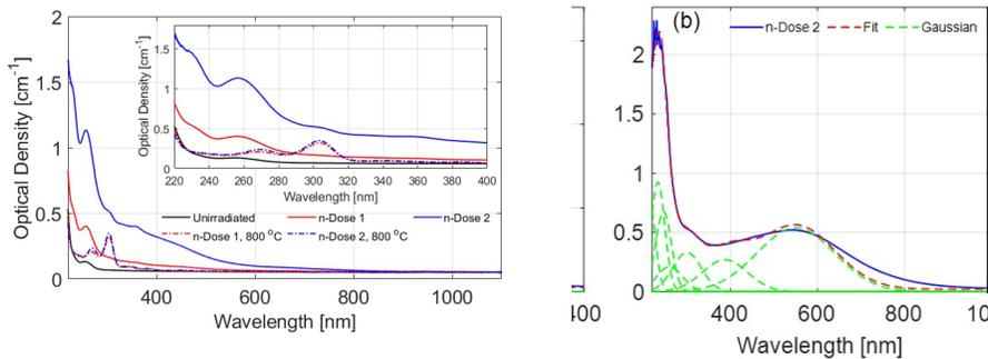
Figure 2. Left: measured sapphire absorption under various annealing conditions. Right: spectral fit to known absorption features in sapphire.
