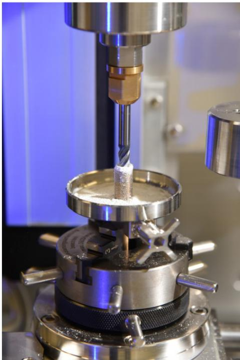
**Defueling module removing surrogate pellet material from rodlet mockup**
