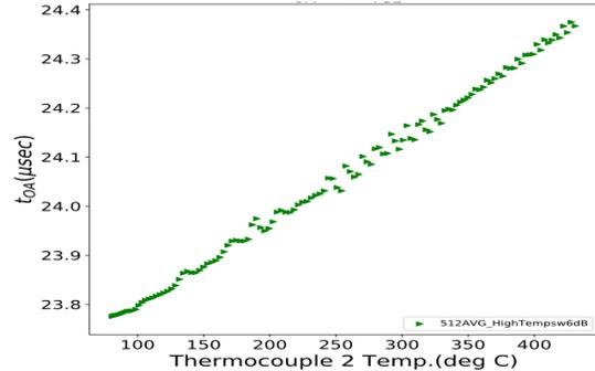
Figure 2. SAW temperature sensor data collection at room temperature to 420 °C.
