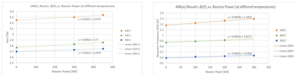
Figure 1. Left: Resonant frequency of the lithium niobate ( $\text{LiNbO}_3$ ) sensor during temperature and reactor power transients. Right: Resonant frequency of the single-crystal aluminum nitride (AlN) sensor.
