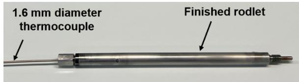
**Finished rodlet with instrumentation installed**
