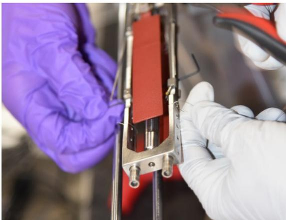
*Figure 1. Fiber optic pressure sensor during the assembly of the fueled experiment.*
