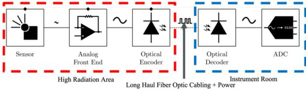
Figure 1. Block diagram of the FREND system.
