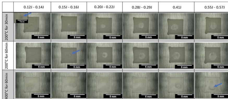
*Figure 1. Determining the threshold laser pulse energy needed to induce failure under three different sintering conditions (i.e., 200°C for 30 min., 200°C for 60 min., and 400°C for 60 min.) at energies between 0.12 J and 0.57 J.*
