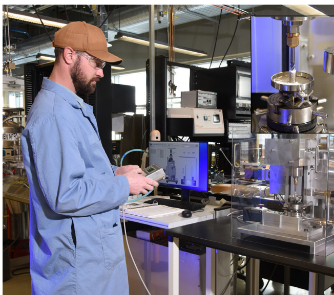
Figure 1. Defueling module removing first pellet from one end of a prototype fuel rod.
