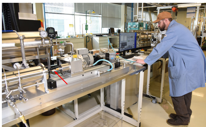
Figure 2. Drilling module starting to drill a 2.5 mm hole 50 mm deep into a fuel pellet stack (in preparation for installing a thermocouple)
