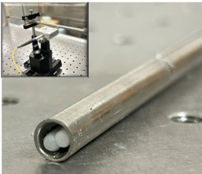
Figure 1. “Laboratory standard” dual fiber optic sensing probe for real-time displacement and strain measurements. Implementation of sensing probe for non-contact monitoring of pipe ballooning shown in the insert.
