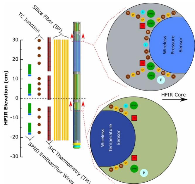
**Figure 2. Schematic showing the instrumentation included in the WIRE-21 experiment.**
