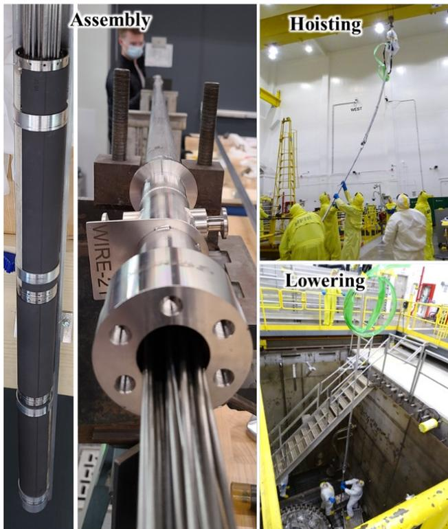
**Figure 3. Pictures of the assembly, hoisting, and lowering of WIRE-21 for insertion into HFIR.**
