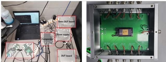
**Figure 2. (Left) MPFD readout system setup in TREAT; (Right) test board with packaged fabricated chip**
