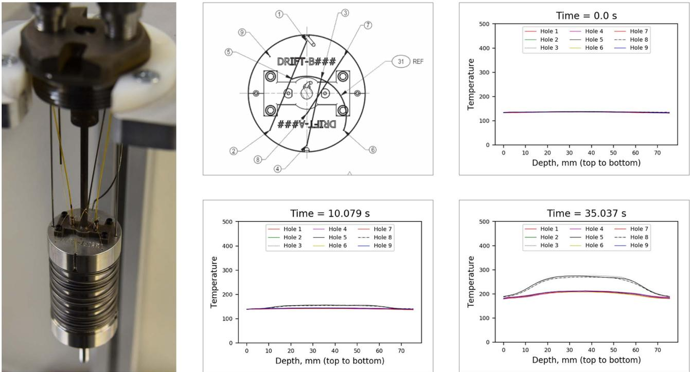
**Figure 2. Photograph of the DRIFT experiment, fiber routing diagram, and three temperature “snapshots” at time = 0 seconds, = 10 seconds after the start of the transient, and = 35 seconds after the start of the transient.**
