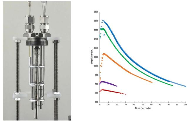
**Figure 1. (Left) photograph of the SETH experiment in TREAT; (Right) summary of the data collected from the fiber-optic-based pyrometry used in that experiment series**
