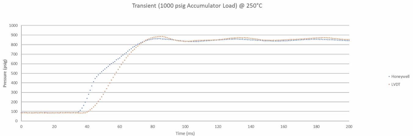
**Figure 2. Transient testing of the THOR LVDT and Honeywell pressure sensors.**
