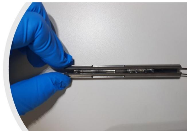
**Figure 1.** LVDT pressure transducer used in the THOR irradiation capsule at TREAT.
