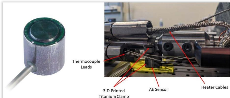
**Figure 1. Acoustic emission sensor (left) and installation on THOR experiment (right).**
