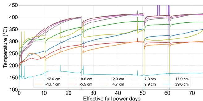
**Figure 4. Temperature recorded from TCs during ~75 days of HFIR irradiation at various locations relative to the core midplane.**
