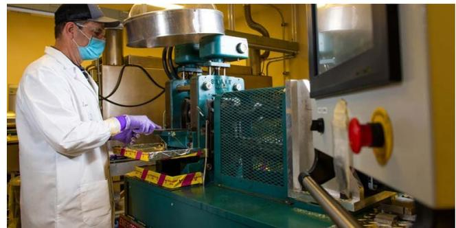
**Figure 3: Rolling mill currently being used to embed fibers within stainless steel for ASI.** This capability is located within the Materials Science and Technology building <https://www.pnnl.gov/materials-science-and-technology-building>
