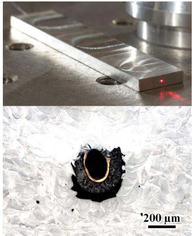
*Figure 4. Pictures of (top) an optical fiber embedded in aluminum via UAM and (bottom) a cross section of a fiber with copper and nickel coatings embedded in stainless steel via LPBF.*
