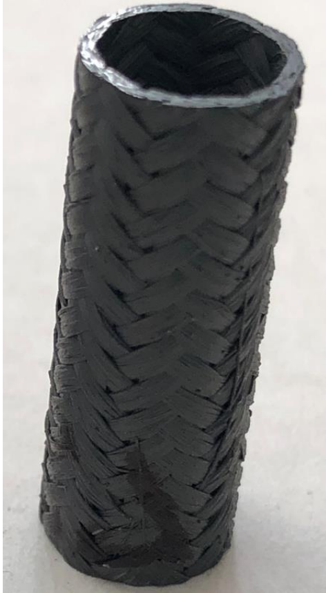
ORNL supplied 1" long SiC/SiC CMC tube samples
