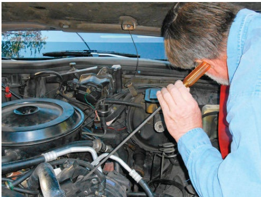
Professional listening for “groaning” of bad coolant pump and smelling for anti-freeze leaks
