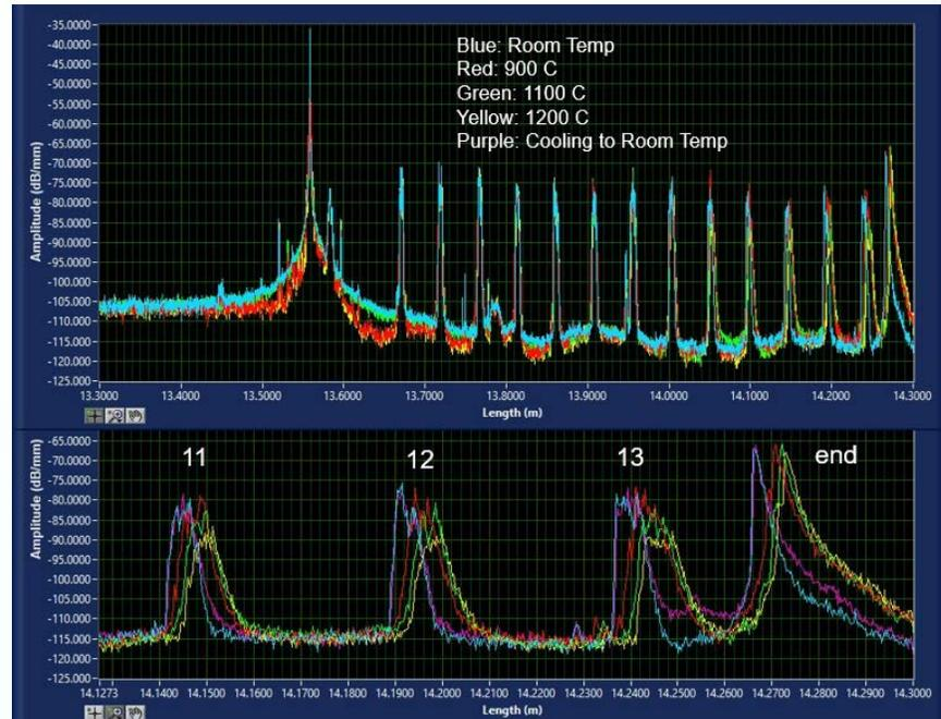
Top: Backscatter profile of sensor #1 before, during, and after the out-of-pile heating from room temperature to 1500°C. Bottom: Top image zoomed in on the last three FBGs in the fiber.
