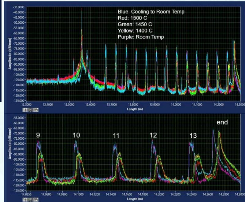
Top: Backscatter profile of sensor #1 before, during, and after the out-of-pile heating from room temperature to 1200°C. Bottom: Top image zoomed in on the last three FBGs in the fiber.
