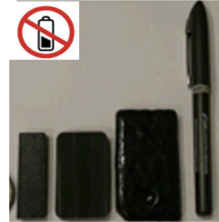
Passive Radiation Hardened RFID Tags
