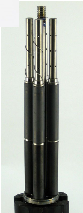
Basic unsealed clad tube capsule
