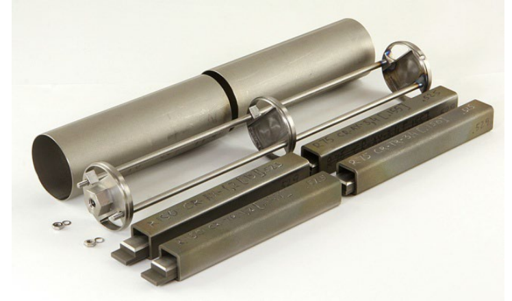
Passively loaded creep test
