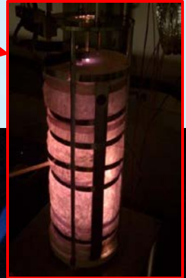
Bench top testing of furnace designed to work with OSU dry tubes
