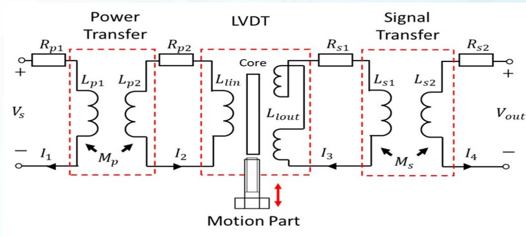
$$V_{out} = j\omega M_s \frac{M_1 - M_2}{L_{lout} + L_{s1}} \frac{M_p}{\frac{(M_1 - M_2)^2}{L_{lout} + L_{s1}} + L_{p2} + L_{lin}} \frac{1}{j\omega L_{p1} + R_{p1} - \frac{j\omega M_p^2}{\frac{(M_1 - M_2)^2}{L_{lout} + L_{s1}} + L_{p2} + L_{lin}}} V_s$$
