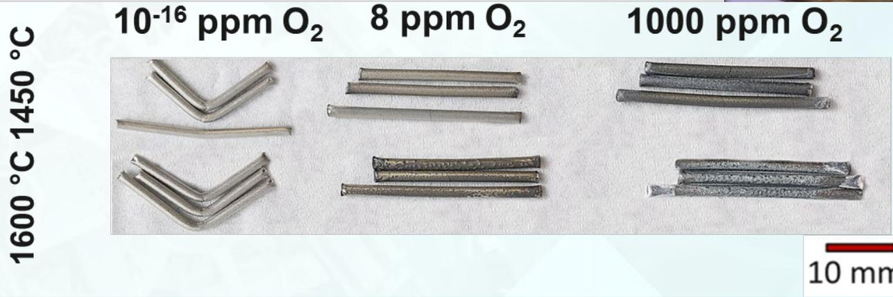
**Finding:** Heat treatment with PO<sub>2</sub> ≥ 8 ppm resulted in Nb sheath embrittlement.
