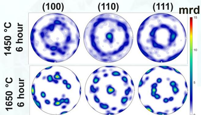
The Nb-P thermoelements do not recrystallize when heat treated at either 1450 or 1650 °C but rather, fiber texture is retained and exacerbated through grain growth.
