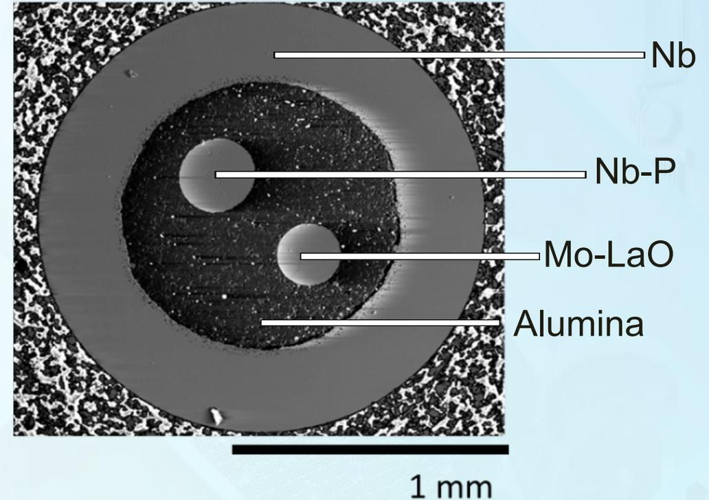
SEM micrograph of HTIR-TC cross-section
