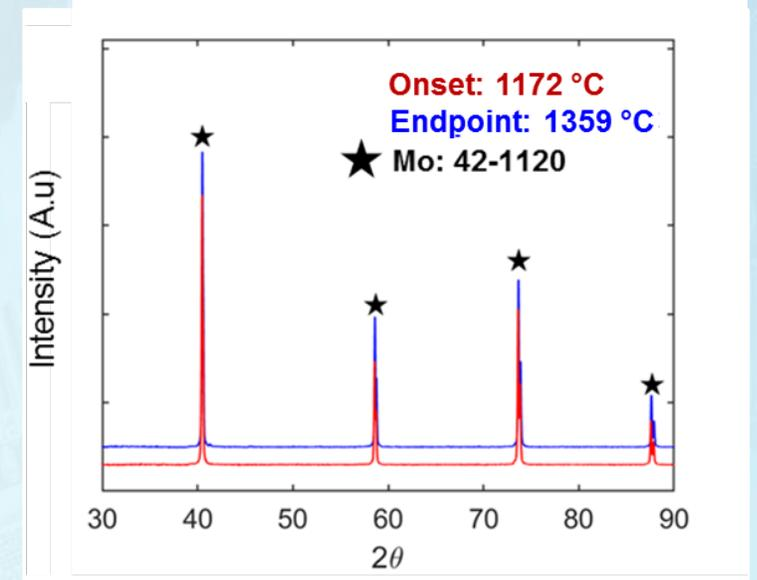
**Findings:** A reversible endothermic reaction occurs in the Mo-LaO thermoelement during heat treatment; however, the Seebeck, electrical resistivity, and chemical phases of the Mo thermoelement remain stable throughout the heat treatment.
