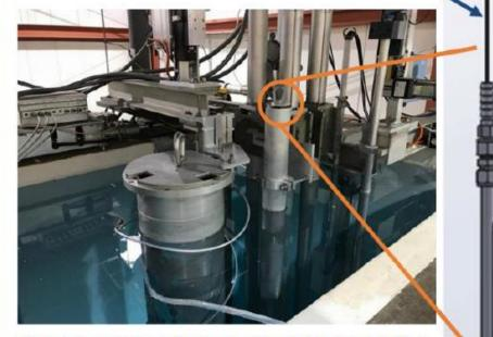
OFBGT installed in the peripheral irradiation facility (PIF) dry tube above the reactor pool of a nuclear reactor
