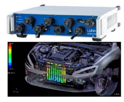
The ODISI 6100 instrument (top), temperature data on a car radiator shown with point cloud visualization.
