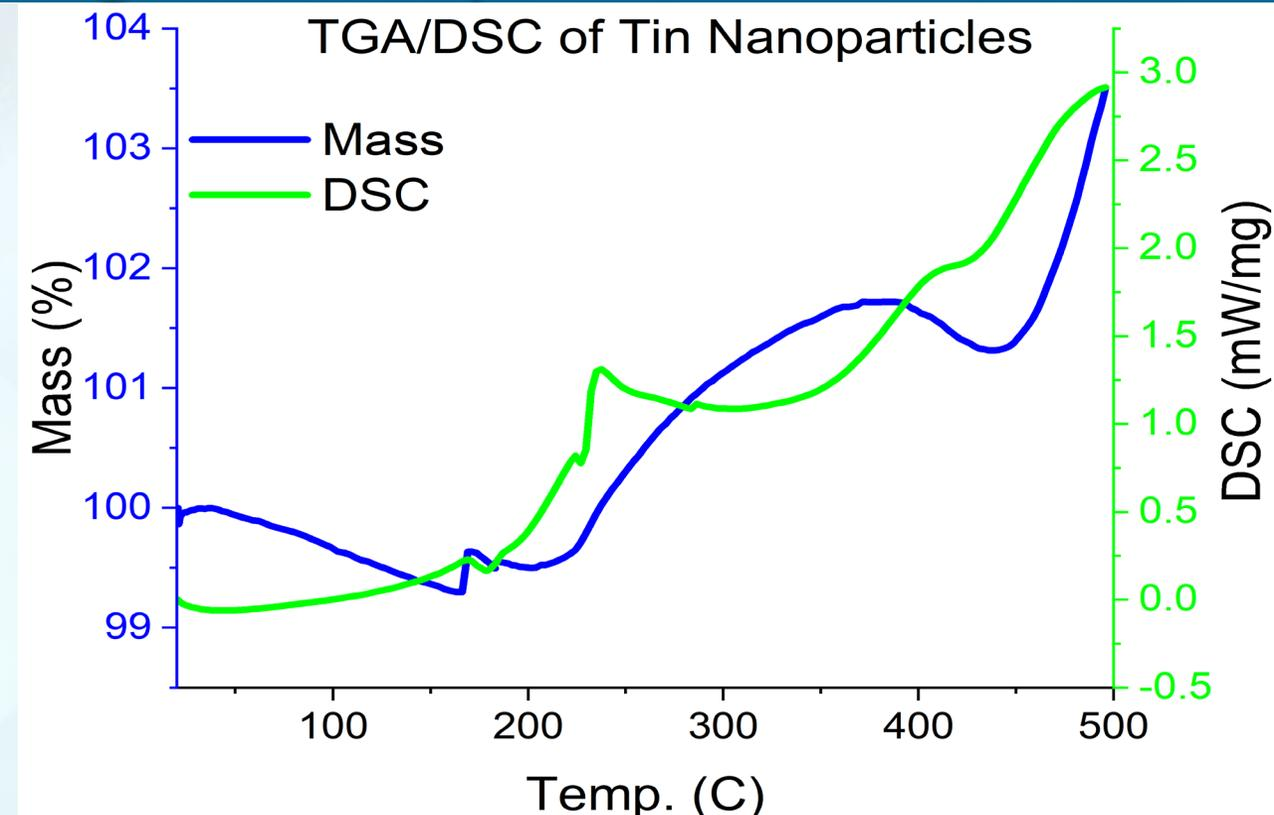
TGA/DSC measurement conducted without an isotherm to estimate PVP content from decomposition. Note, the sample gained mass as the sample was heated to 500°C.
