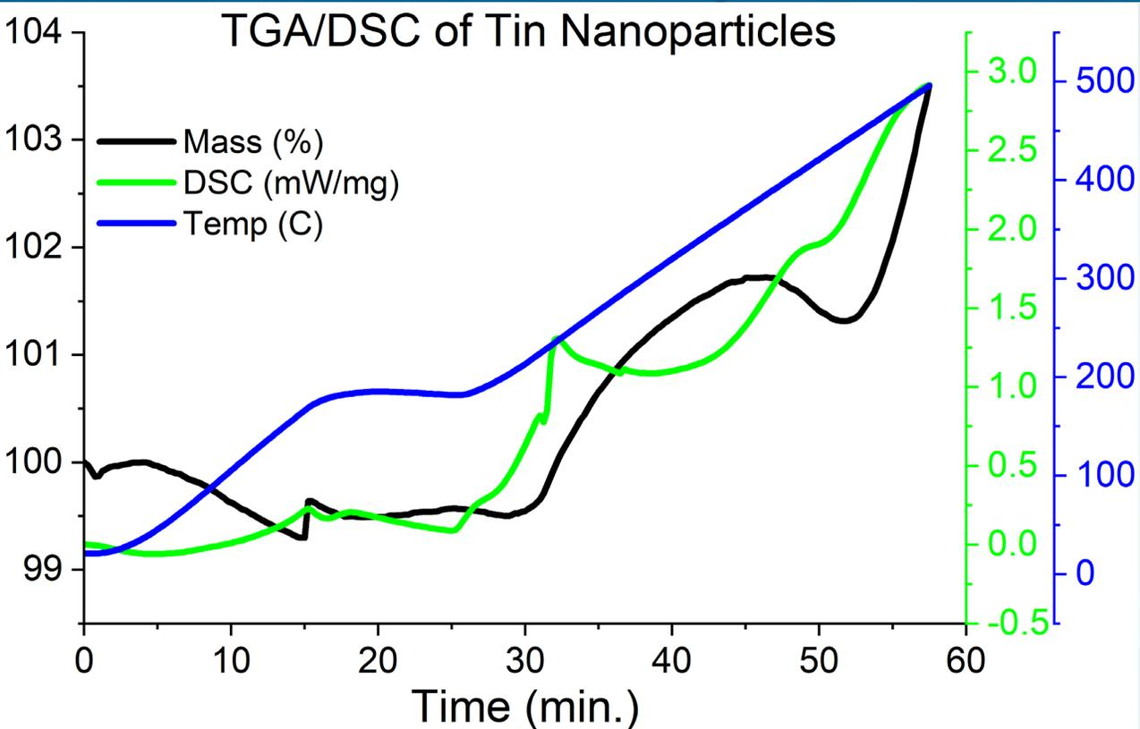
TGA/DSC measurement conducted with an isotherm at 175 °C for 10 minutes (Melting Point at ~150 °C)
