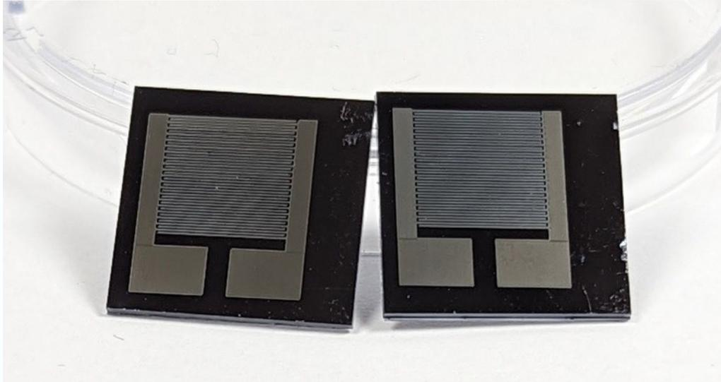
IDEs printed with Tin nanoparticle ink on additively manufactured alumina container.
