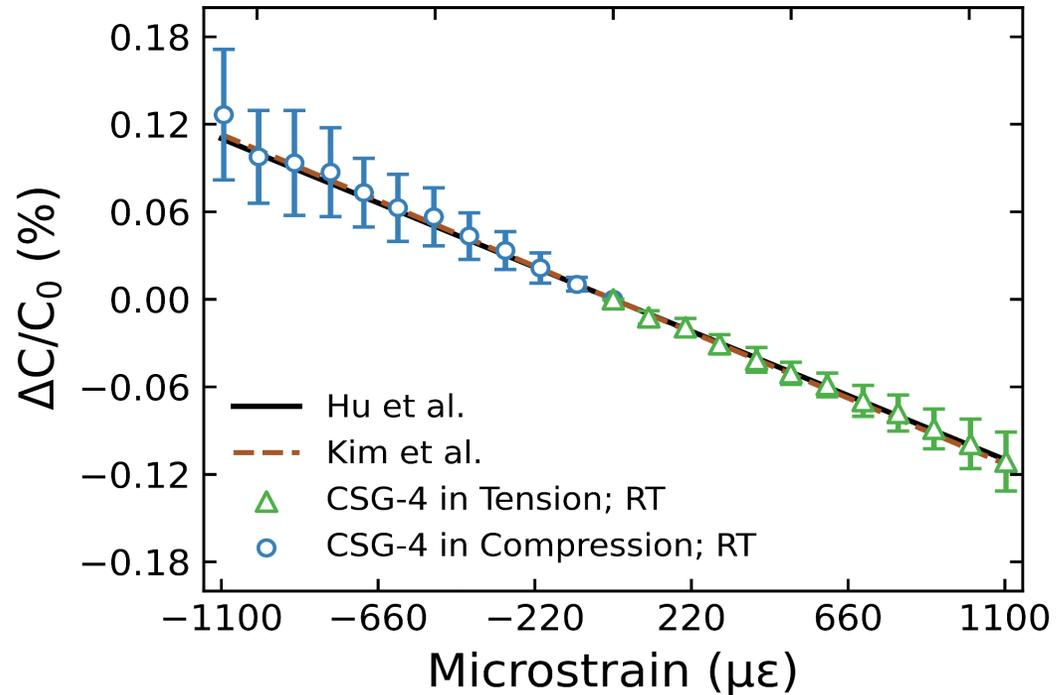
Printed strain gauge output in both compression and tensile mechanical strain
