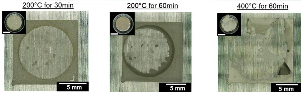
Example of pull-off adhesion samples that failed at the substrate/film interface for each sintering condition
