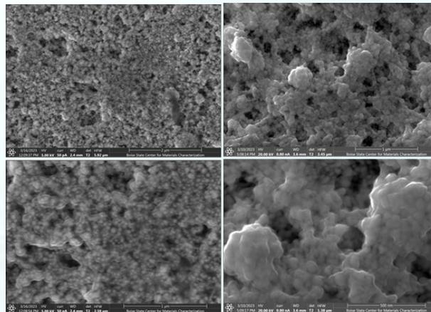
Printed sample      Thermal sintering at 350°C – 30 minutes
