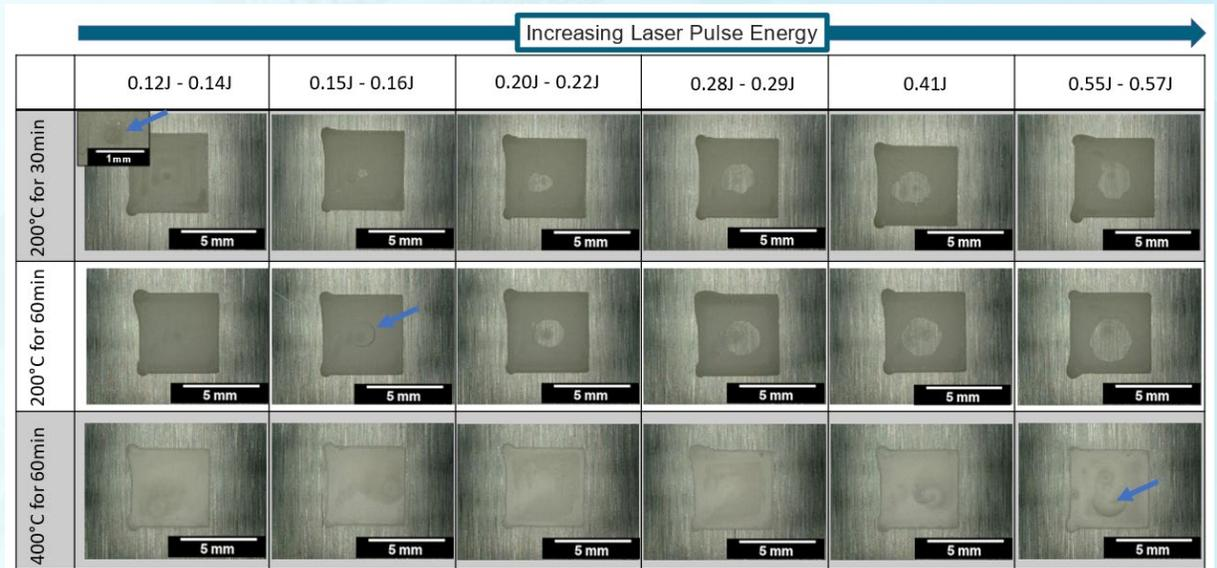
Results from monotonically increasing the laser pulse energy for samples sintered at three different conditions; arrows indicate onset of failure
