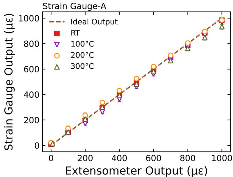
Strain gauge output against a calibrated extensometer
