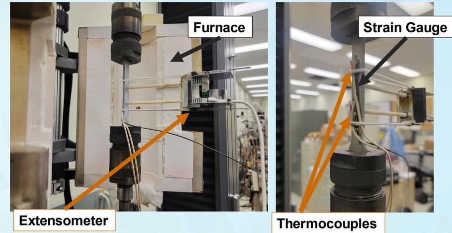
Strain gauge loaded in axial mechanical test fixture
