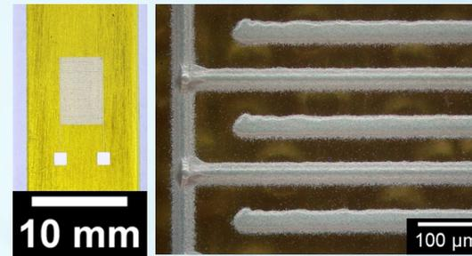
Strain gauge fabricated using aerosol jet printing
