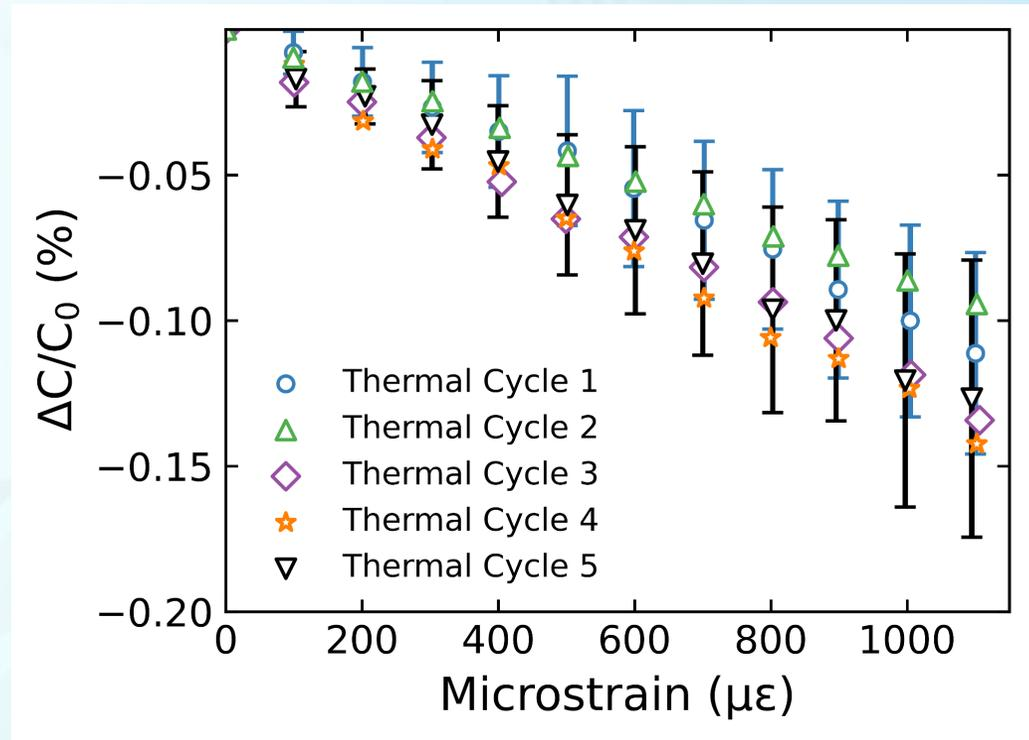
Sensitivity of printed strain gauge after thermally cycling up to 300 °C
