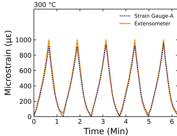
Results from cyclic testing at up to 1000  $\mu\epsilon$  at 300 °C
