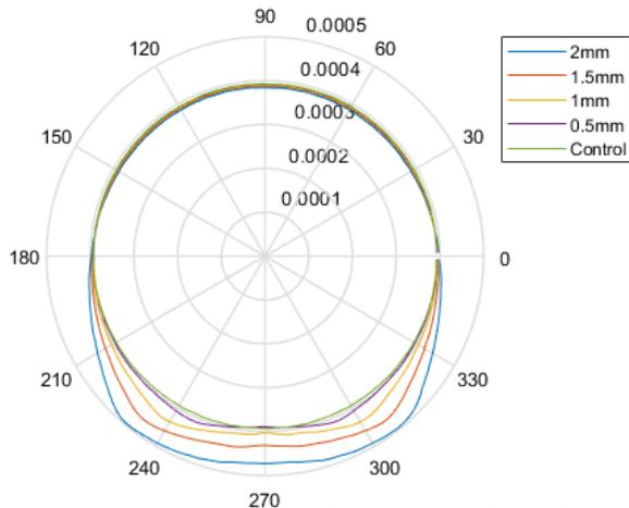
FEM strain predictions for Axial (top) and Hoop (bottom) strains at center of mockup
