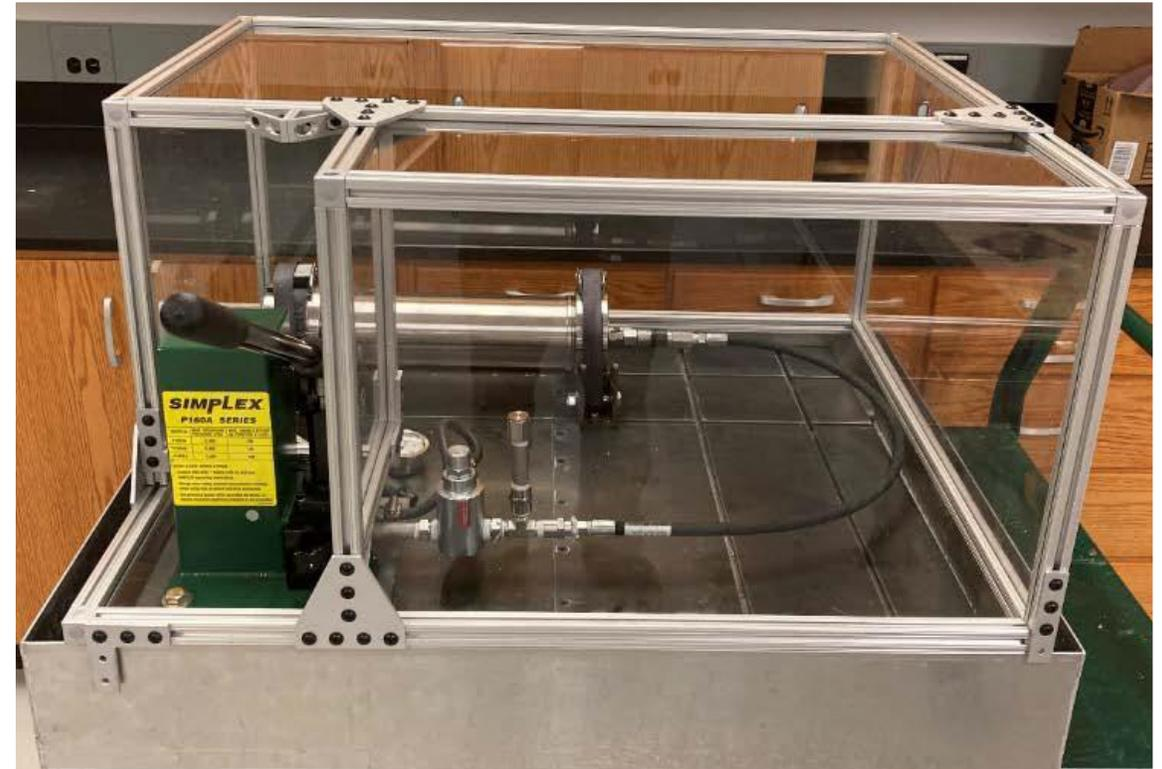
Test bed for studying feasibility of strain-based FFS
