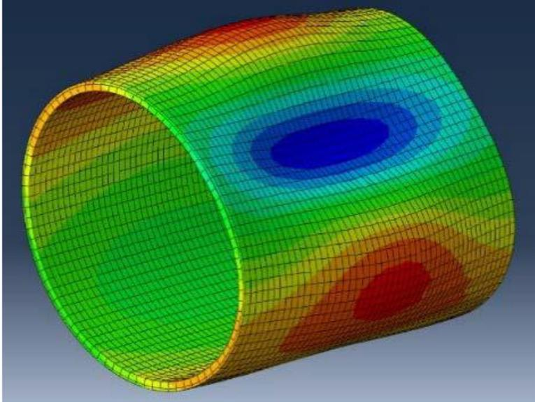
Exaggerated Deformation Profile Prediction
