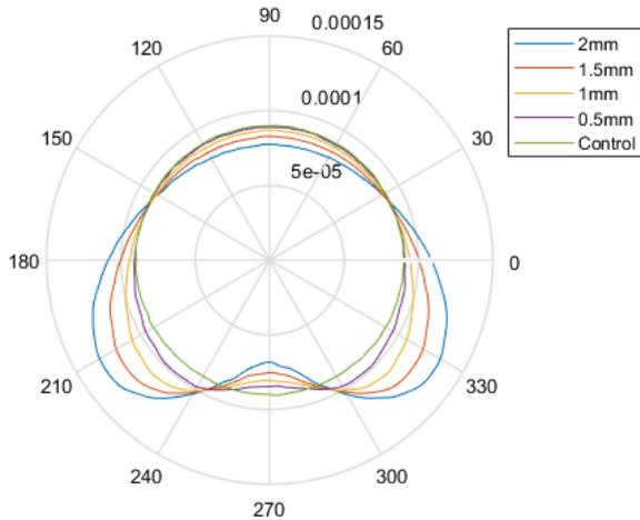
Superimposed Hoop Strain Profiles at Center Position
