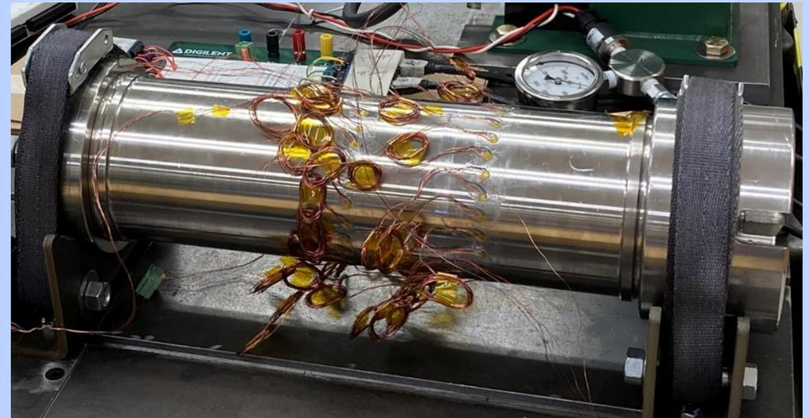
Pressure tolerant mockup for feasibility testing
