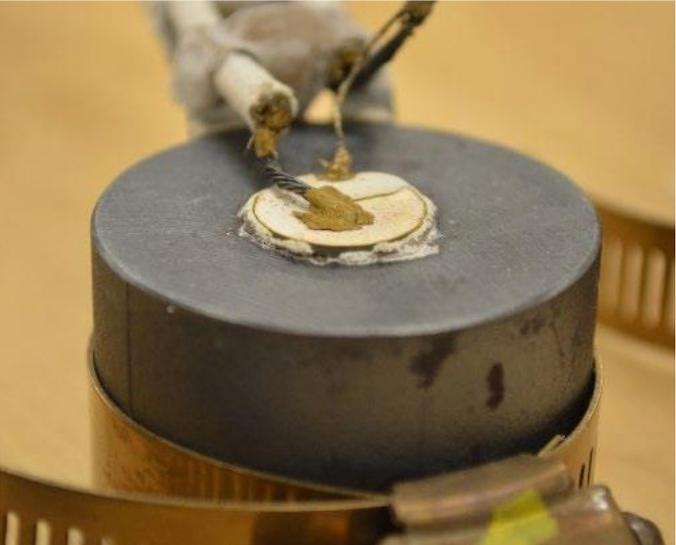
Example sensor setup for live thermal testing
