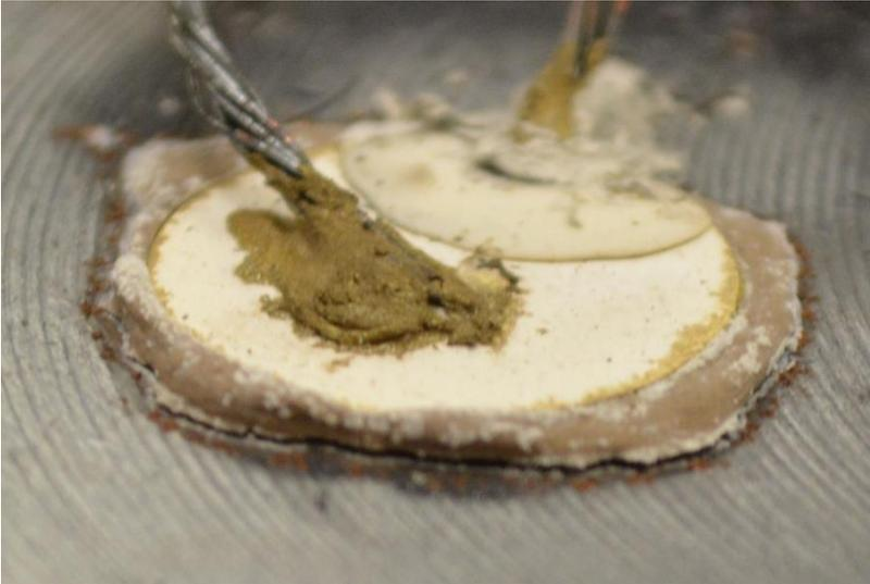
Failed adhesive (cracking on substrate surface)
