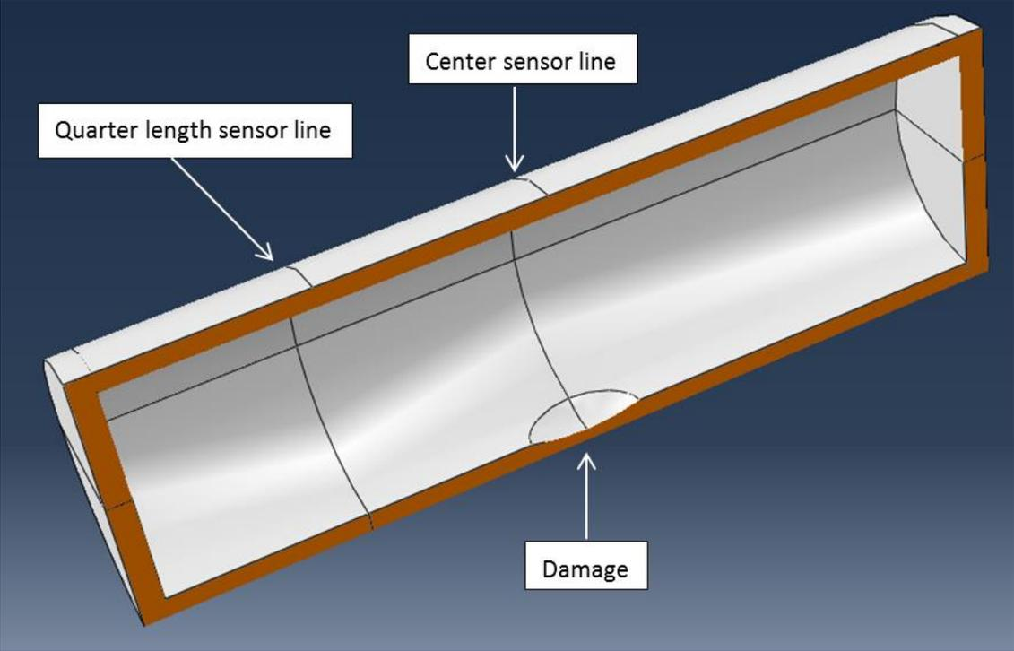
CAD model of example damage showing simulated strain sensor extraction regions
