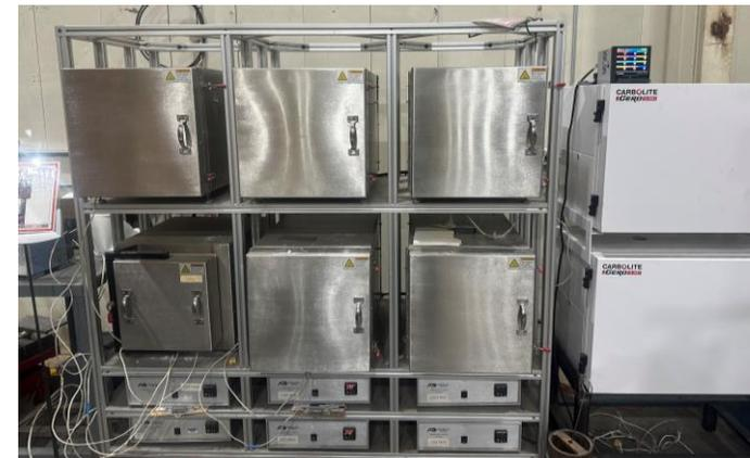
Box furnace battery (1200 °C)
