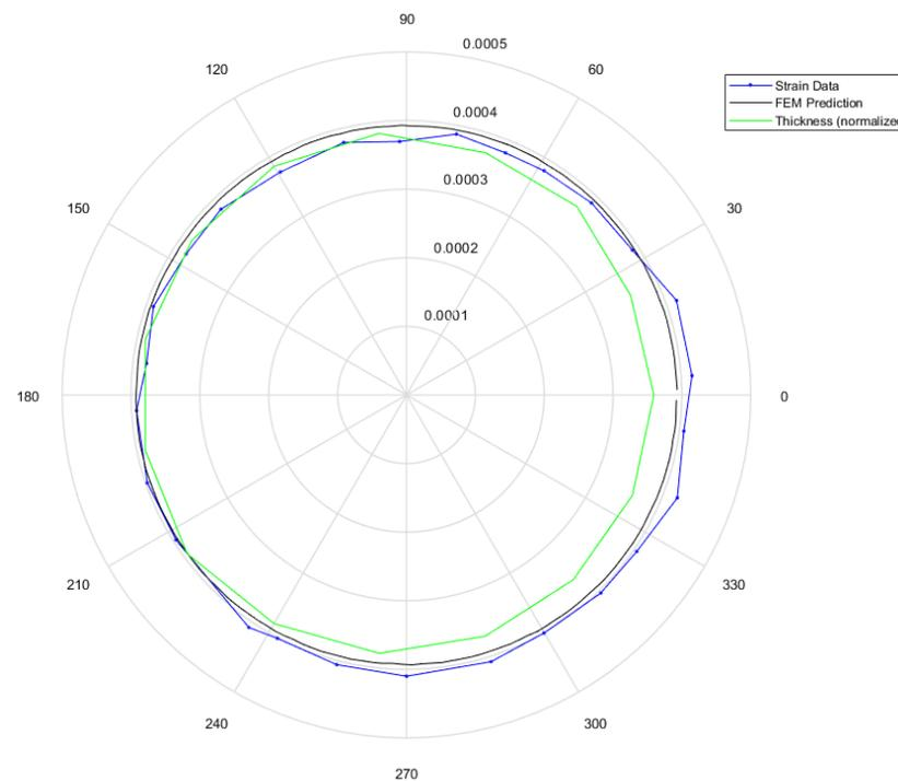
Control mockup strains with superimposed wall thickness measurements (normalized)
