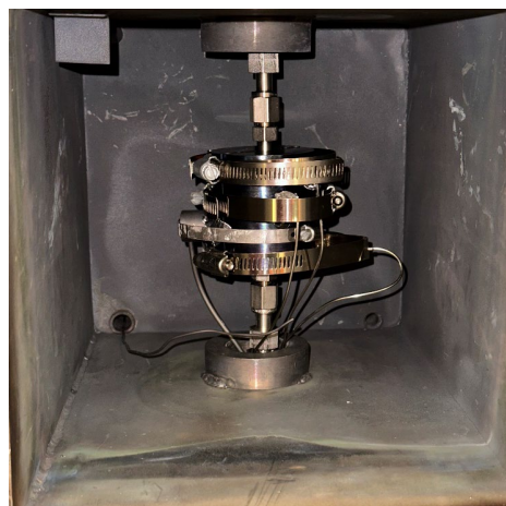
Experimental setup in furnace with hose clamps securing sensors to heat sink
