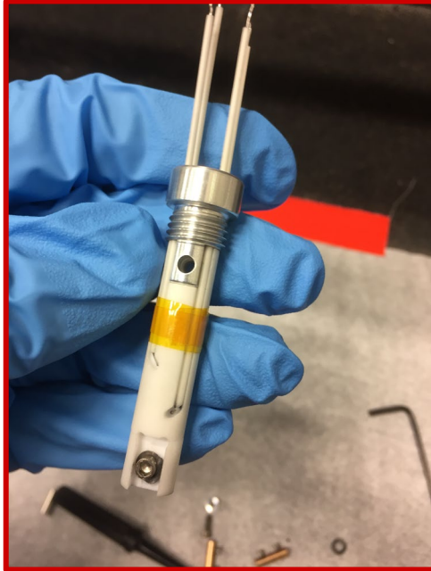
Alumina sample holder developed for real-time electrical monitoring (fit test prior to final integration)
