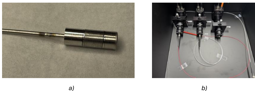
Figure 12: (a) Photograph of updated fiber optic pressure sensor. (b) Photograph of the photodiode-based high-speed pyrometry system.
