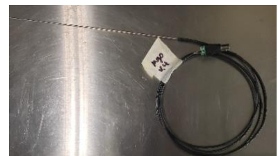
Figure 3: Prototype SPND fabricated at INL
