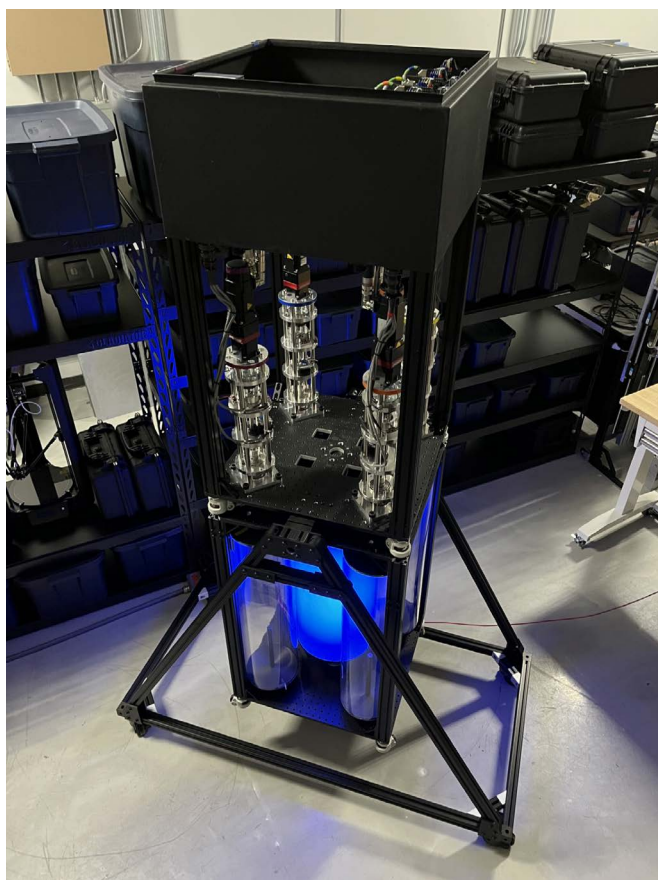
Figure 3. MACS with actuator cell and surrogate reactor cell.
